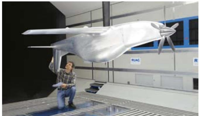
The wind tunnel test campaign covered more than 1000 polars most of which were in a power-on configuration. During two extensive test campaigns, the model and its instrumentation performed flawlessly, allowing the test to be performed on schedule and giving the customer perfect satisfaction.
