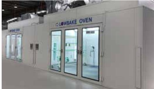
inlet filtration and are sealed to prevent dust inclusions impacting paint finishes. Lighting has also been configured to provide in excess of 1200 lux at the working surface. The paint booths are temperature-controlled (both heating and cooling) and have a full downdraught configuration providing the best performance for paint overspray removal.
