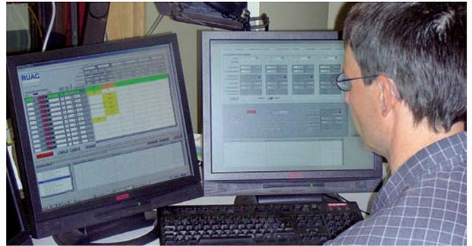
The teach-in feature of the AP-Player is especially useful for ground effect tests with the rear model support. With one mouse-click the current position can be copied into the current position sequence; instead of entering the information numerically the model can be moved manually to the desired position and the automatically measured numerical value at this position is inserted.
