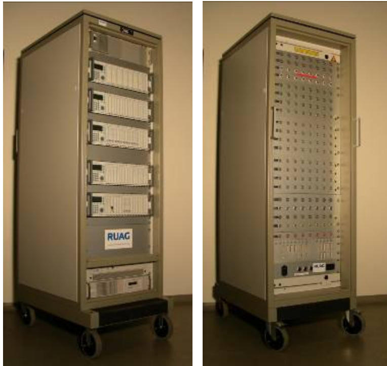
Fig. 2: Data acquisition systems in wind tunnels at RUAG Aerospace, with MGCplus technology: Front (on the left) and back with connection boards (on the right)
