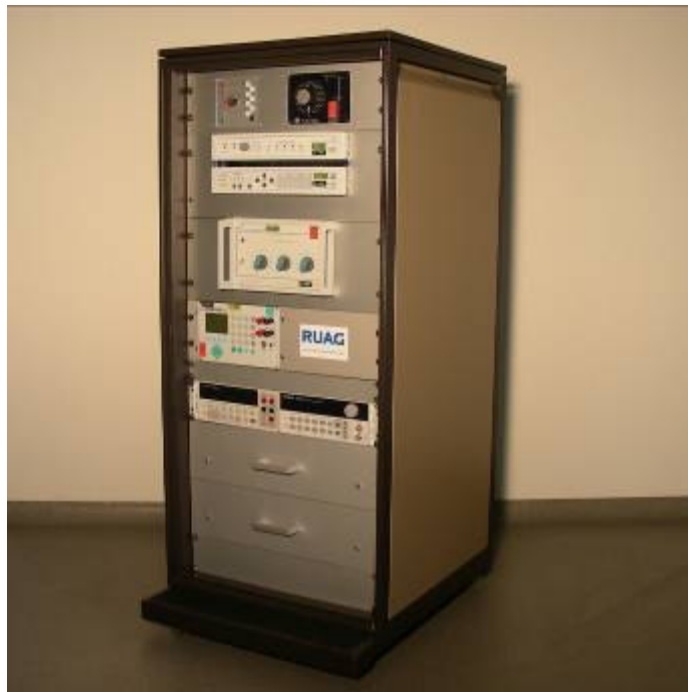
Fig. 3: Calibration tower at RUAG Aerospace for wind tunnel data acquisition systems
