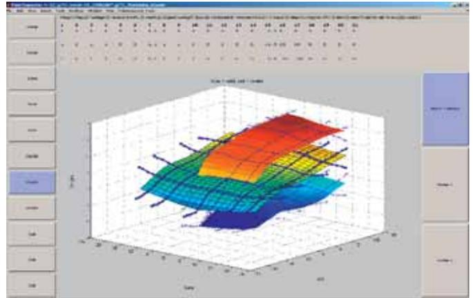
Screen shot of the **PolarInspector** showing maps for the pitching moment for three elevator deflections over angle of attack and sideslip.
