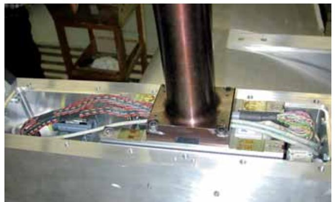
Central wing and balance interfacing the model support
