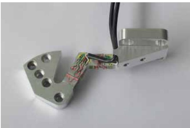
Strain gauge instrumented flap hinge and calibration of hinge moments
