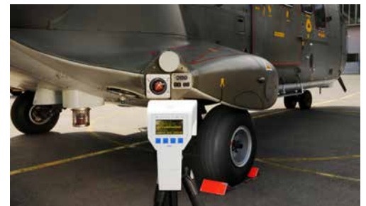
Using missim to test a helicopter's EW system
