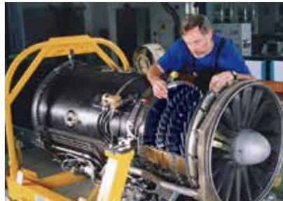
Inspection of FAN rotor
