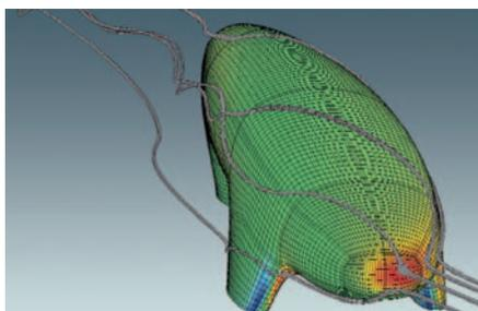
Wind tunnel tests were conducted at ETH in Zurich and in the Automotive Wind Tunnel (AWTE) using the rolling road feature. CFD simulations were performed using the Navier-Stokes Multi Block Solver NSMB.
