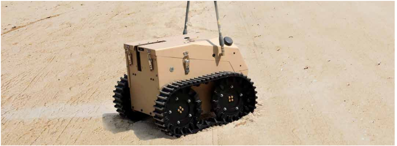
Scopus 200 robotic platform with tracks and without target lifter and target.
