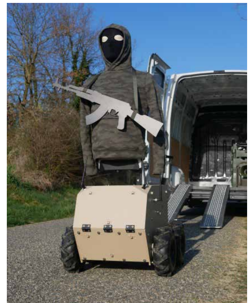
Scopus 200 with 3D target and mock-up rifle dismounting from transport vehicle.
