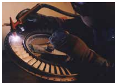
Turbine nozzle - Stage 1 welding
