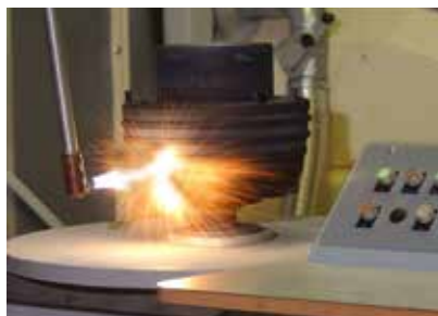
Compressor rotor rear spool coating/thermal spraying
