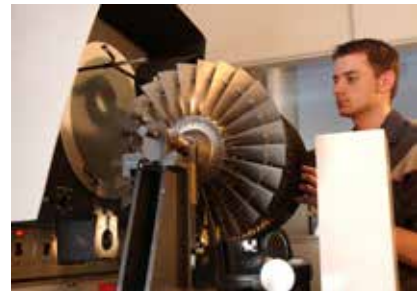
Compressor rotor measurement
