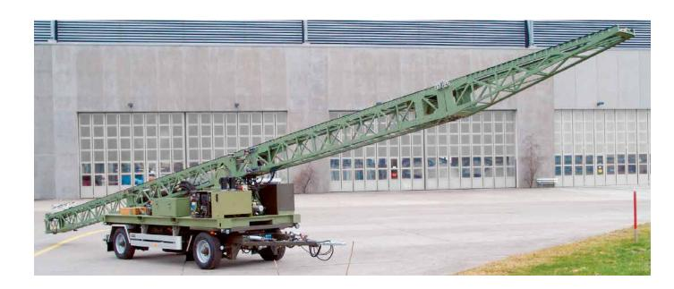
A launching device for unmanned aerial vehicles (UAV), specifically developed by RUAG Aviation, allows for full operational flexibility in the deployment of UAV. The DC4 launcher features a compact design for easy manoeuvrability, is self-contained and operates independently of external power sources. The unit proves reliable, simple to maintain and cost efficient.
