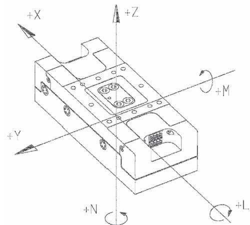
**Figure 3. Coordinate system for block-type balances.**
