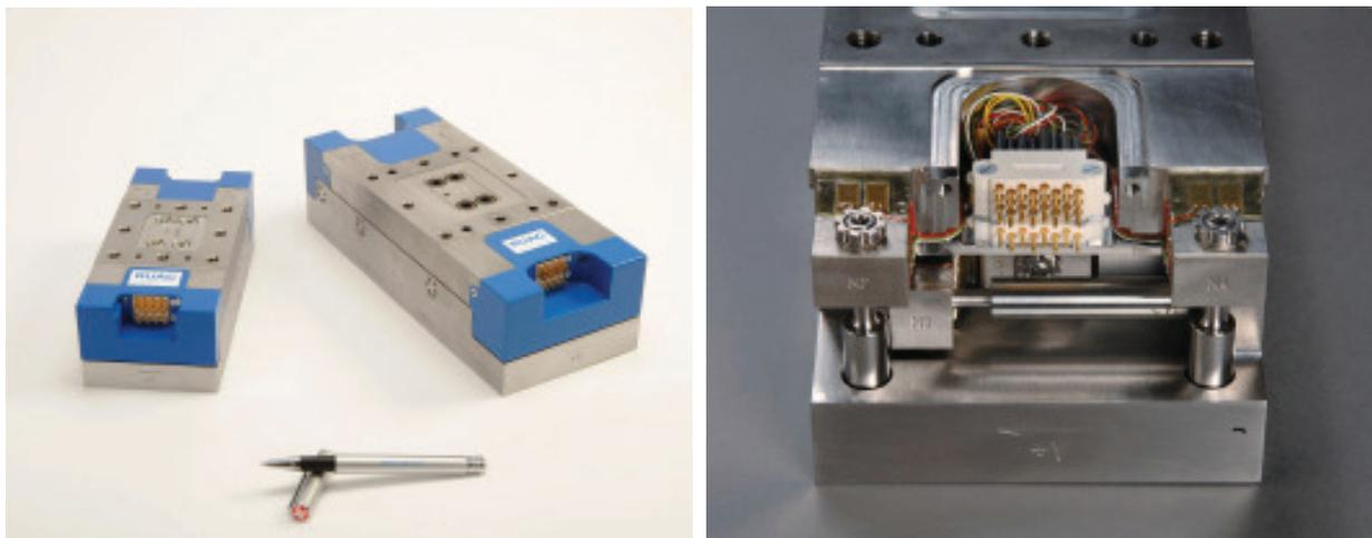
**Figure 2. RUAG Balance family 7xx with its characteristic blue protection cover (796 to the left, 788 to the right). The frontal view shows the non-metric part with one lateral and two vertical measurement elements. The forces are transferred by joint-rods from the lower metric end. Between the vertical elements the extremely rigid and reliable electrical plugs are visible.**
