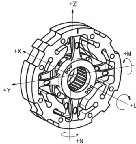
**Figure 5. Coordinate system for rotating shaft balances.**
