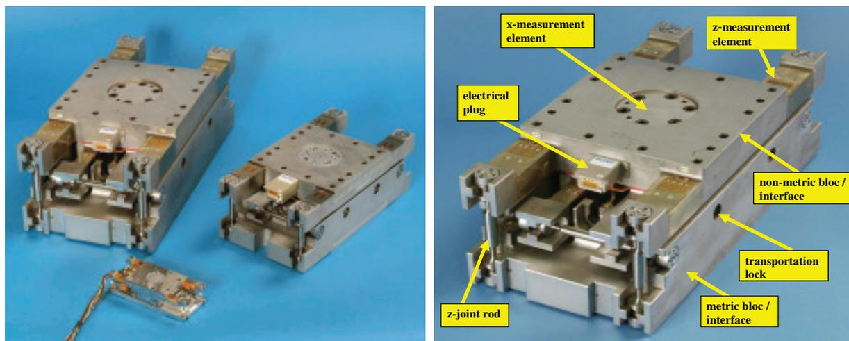
**Figure 1. RUAG Balance family 1xx. The load envelopes are ranging from 20 to 12'500 N (axial force) and 10 to 25'000 N (normal force), the dimensions (l x w x h) from 100 mm x 25 mm x 22 mm to 540 mm x 260 mm x 230 mm, and the balance mass from 0.25 to 180 kg. The view to the right shows the main components of the balance and the measurement elements with their parallel beams.**
