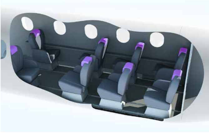
Standard cabin layout for 8 passengers
