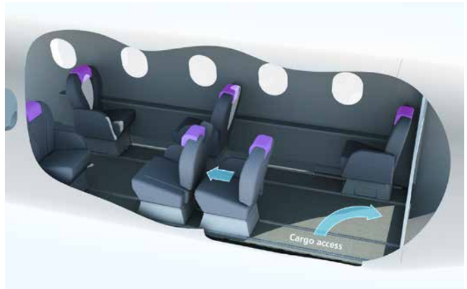
Optimised cabin layout for 6 passengers
