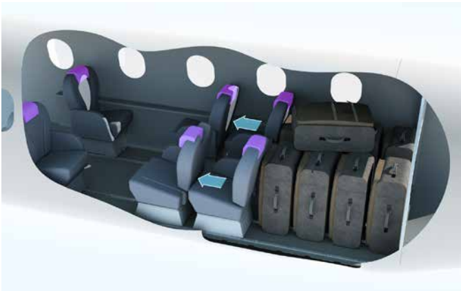
6 seat cabin layout optimised for 4 passengers and cargo
