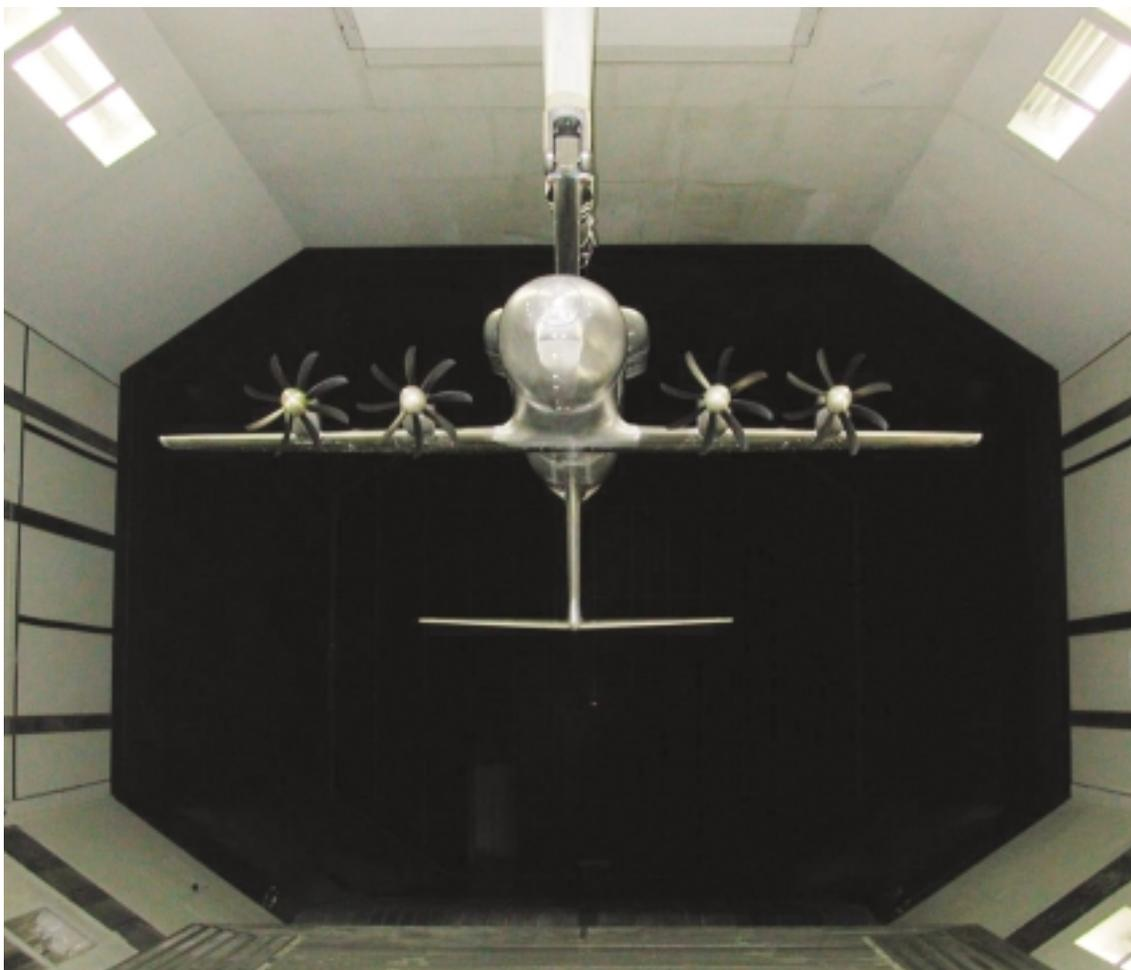
A400M, 1:15 scale wind tunnel model
