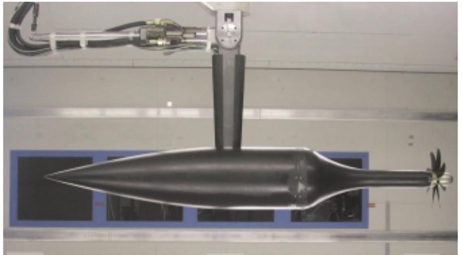
Minimum Body test setup in the wind tunnel
