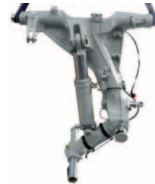
Do 328 landing gear prepared for the shock absorber qualification test
