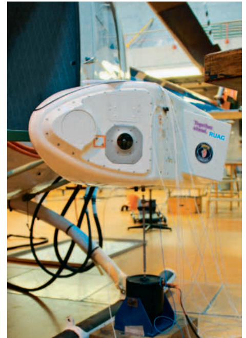
RUAG developed self protection pod on the Bell 205 being subjected to modal investigations.
