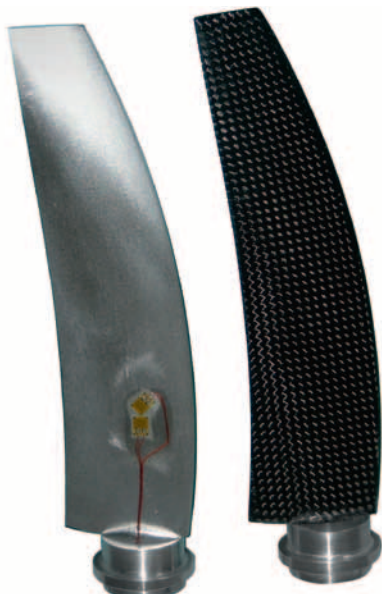
An aluminum and carbon blade, designed by RUAG for a counter rotating open fan propulsor
