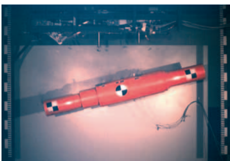
Ground based store separation test for the nEUROn pantograph release mechanism.
