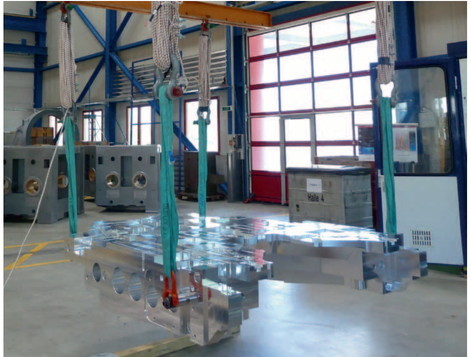
Modal characteristics test on the 1.6t wafer stage metro frame
