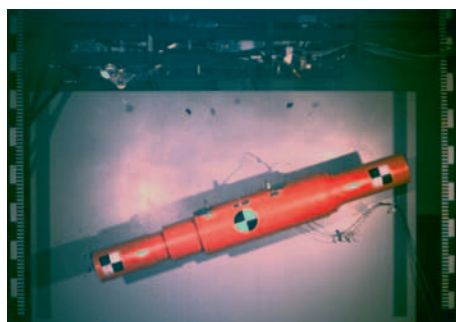
Ground based store separation test for the nEUROn pantograph release mechanism.
