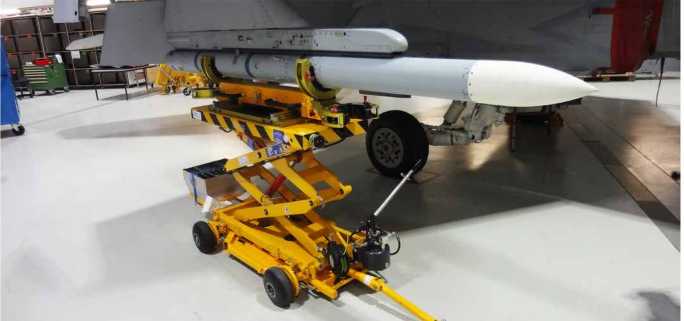
Transporting, positioning, loading and unloading missiles and Flight Profile Recorder on F/A-18 C/D military fighter aircraft for all wing stations is a straightforward and compact task when you rely on RUAG Aviation's ground support equipment. The RUAG Missile Loader Wing Stations (MLWS) enables the loading of different types of missiles with minimum handling and maximum flexibility. This MLWS is also a smart and effective solution for meeting employee health and workplace safety regulations.
