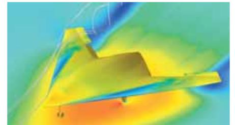
If necessary, a further low-speed wind tunnel test campaign will take place early next year to clarify final details. On the CFD side, additional simulations using a more detailed external geometry will be performed. The simulations will also be used to gain some additional insight into the results obtained during the ground effect tests in the wind tunnel (for example the effect of the floor boundary layer will be studied).
