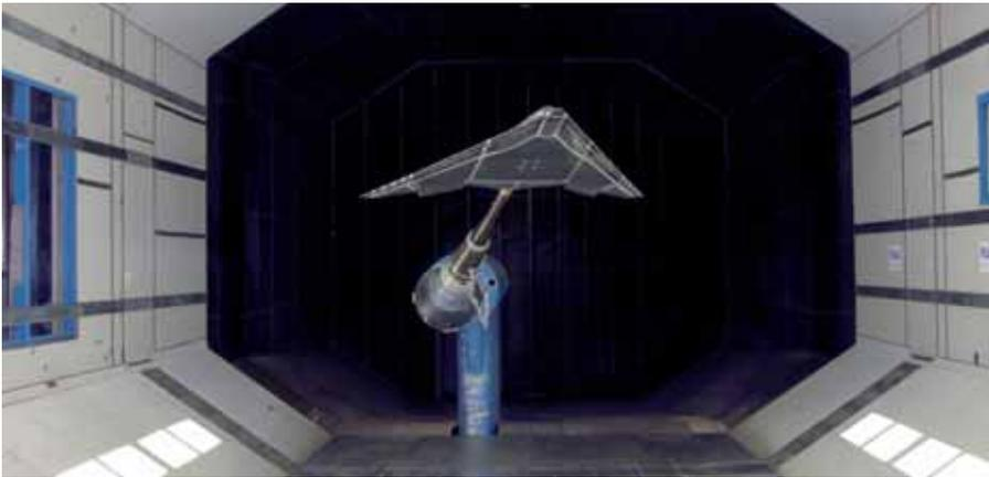
Campaigns with a larger model (1:5) followed. One low-speed campaign was mainly dedicated to the study of ground effect. For this, an intermediate floor is installed in the test section of the LWTE. The model is mounted through a dorsal strut to the rear model manipulator (REMOS). This setup allows to quickly measure a wide range of angles of attack, sideslips and heights above the floor. The results were found to confirm the data previously obtained from the CFD calculations.
