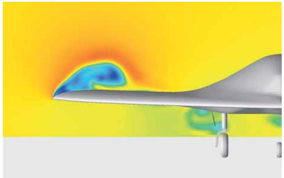
The results were found to be satisfactory and in a second step the actual geometry of the nEUROn was modeled. The simulation matrix included various angles of attack and sideslip, and altitudes over the ground. Due to the unconventional aerodynamics, a good understanding of the effects is of prime importance in order to assure a safe take-off and landing. For this reason, it was decided to confirm and complement the theoretical results by wind tunnel tests.
