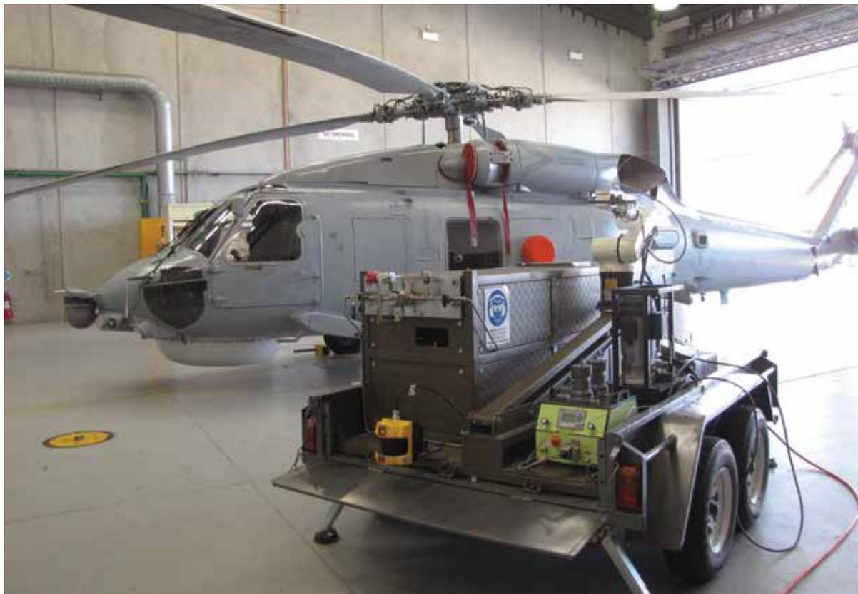
The RAN's Seahawk helicopters have seen SPD repairs (mobile SPD unit pictured) used on non-structural parts since 2009.
