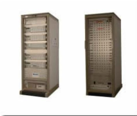
*Fig. 4: Data acquisition system with MGCplus technology: Front (on the left) and back with connection boards (on the right)*
